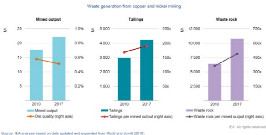
Figure 5 - Evolution of waste generation and ore quality from copper and nickel mining between 2010 and 2017 6
