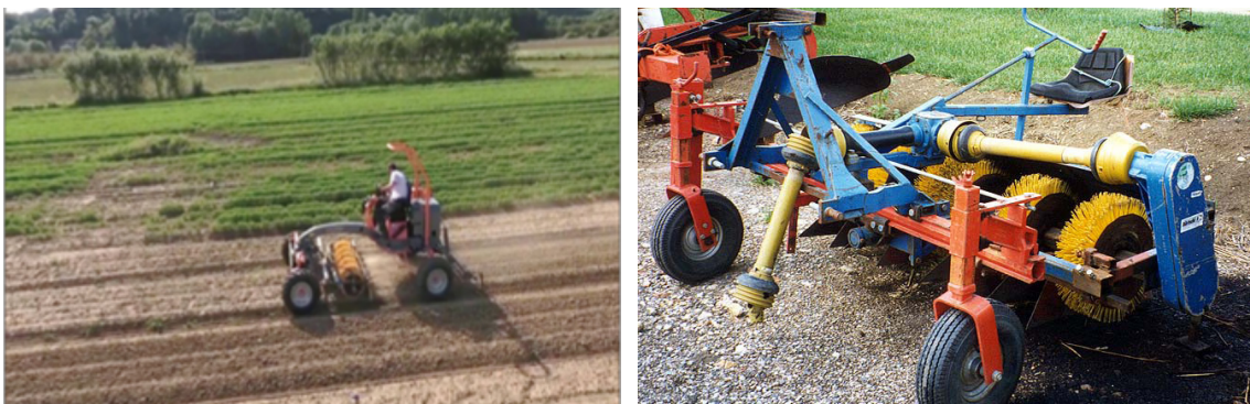
Figure 24. The horizontal axis brush hoe (left: mounted on a specialised tool-carrier tractor)
